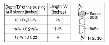
6 Remove the backing from the support blocks and attach them to the inside of the wall sleeve as shown FIG 37. Slide the baffle into slots of the support blocks
